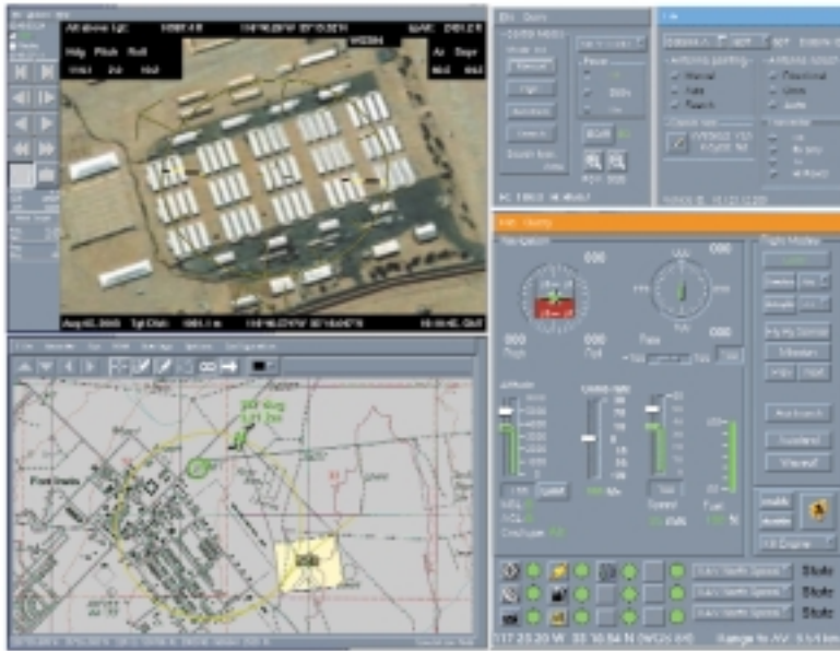
Screen shot of CDL Systems' Vehicle Control Station (VCS) software for STANAG 4586, the NATO UAV Interoperability standard.
